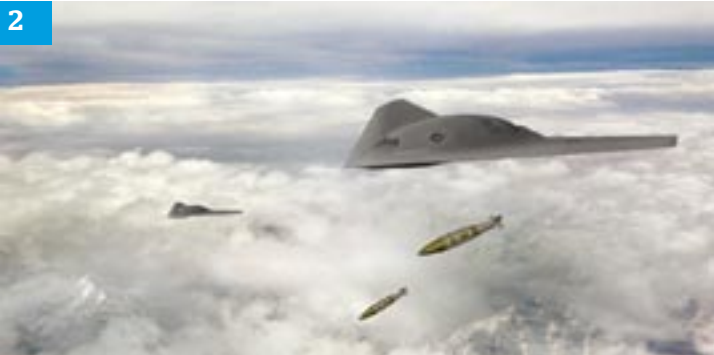
JDAM (Joint Direct Attack Munition) release from the J-UCAS (Joint – Unmanned Combat Air System) X-45C air vehicle. © DARPA
