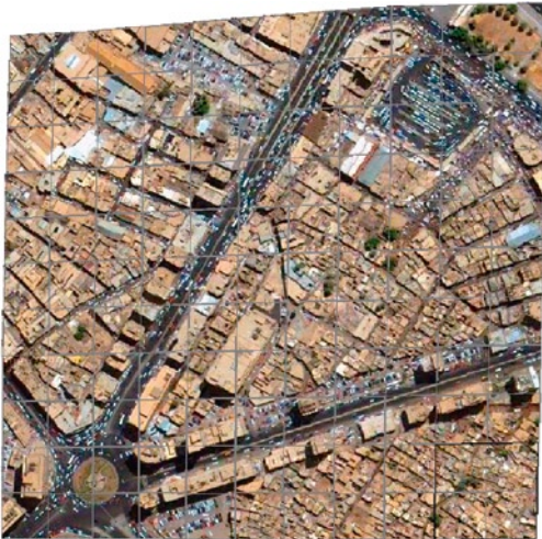
After bundle adjustment. Using homography for image content mapping – a) before and b) after bundle adjustment.
