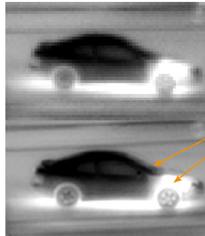
(top) IR sensor image (41 by 71 pixels); (bottom) TRE result for a target tracked as it moves within the sensor FOV.
